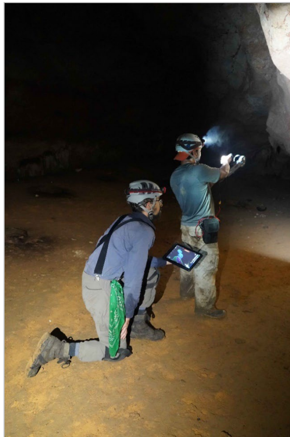
Figure 4. Scanning with the Hovermap (Gonzalo Pleitez and Shane Montgomery pictured) Photo courtesy of the LCAR.
