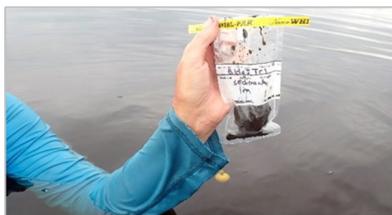
Figure 4. Photograph of an example of collecting marine sediment in a sterile whirl-pak at Ek Way Nal. Photograph by Cher Foster.
