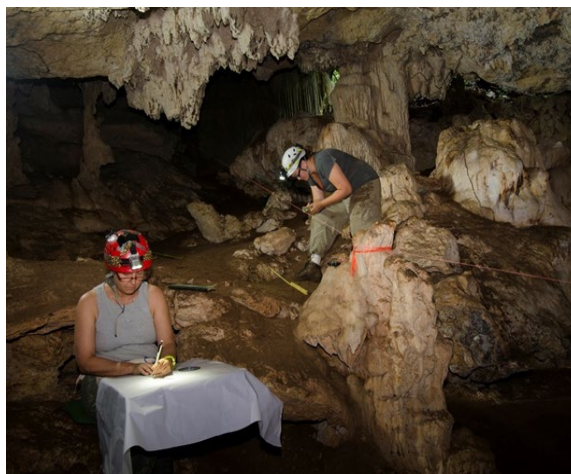
Figure 2. In field cave mapping using baseline offset method (Holley Moyes and Erin Ray pictured) Photo courtesy of the BCRP.
